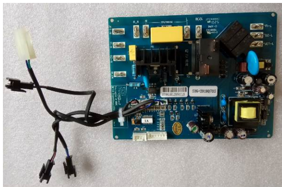
Main Power board (PCB)
